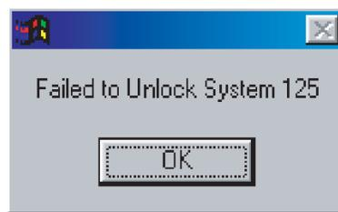
The "Failed to Unlock System 125" message means that the Cannondale Diagnostic and Maintenance Tool was not able to communicate with the vehicle ECU. There can be several causes:
